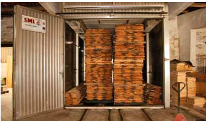
TIMBER DRYING KILN SILVINO LINDO, 40 M 3
